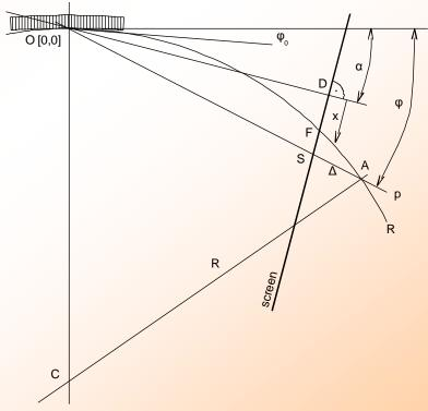
Rowland geometry in imaging spectrometer.
