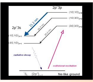
Pump: 300-ps laser pulses, wavelength 1.3  $\mu$ m Weak prepulse (<10<sup>11</sup> Wcm<sup>-2</sup>) applied 10 or **50 ns** ahead of the main pulse Main pulse produces ~4x10<sup>13</sup> Wcm<sup>-2</sup>
