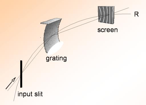
Reflection grating EUV spectrometer with the slit, torroidal grating and BI CCD detector placed on a Rowland circle.
