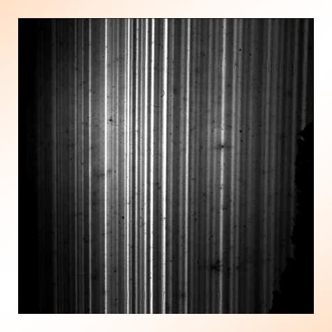
BI CCD image of time integrated spectral lines in the range from 10 nm to 30 nm (Nitrogen filled capillary). Wavelength is on horizontal axis and space coordinate along the input spectrometer slit is on vertical axis.
