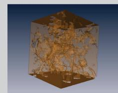
Microtomographic image of sandstone rock microstructure
