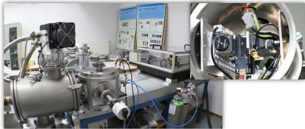
Photograph of the EUV source, microscope chamber and pumping laser.
