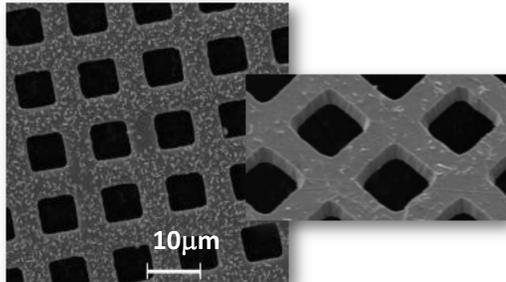
Mesh ~4μm thick, ~11xDOF
