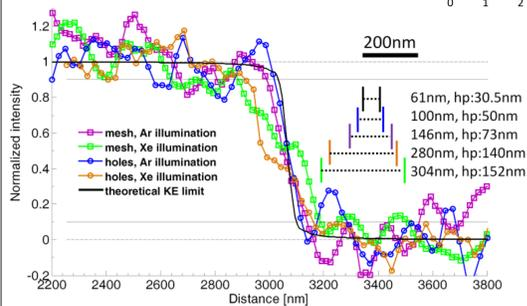
Typical KE lineouts indicating 10-90% intensity transition in the EUV image related to Rayleigh resolution criterion for both objects and different illumination bandwidths and the theoretical KE limit.
