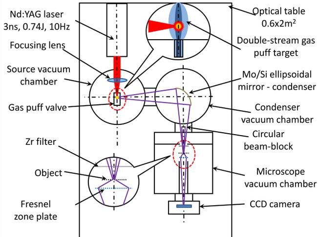
Scheme of the EUV microscope based on a laser plasma EUV source.
