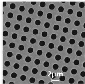
Hole pattern 70nm thick 10nm carbon foil + 60nm Au for optical contrast, ~0.2xDOF
