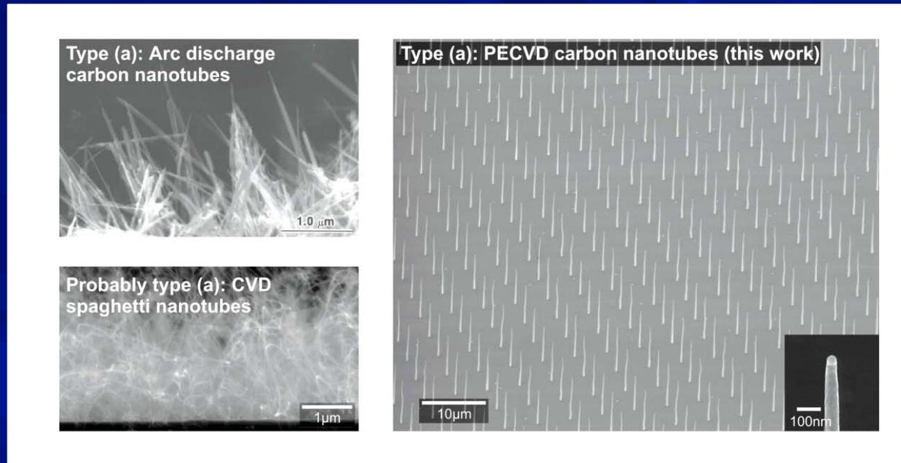
In order to design and fabricate cathodes with optimized performance, it must be taken into account that when several emitters are assembled to form an array, an electrostatic screening effect appears between the emitters.
