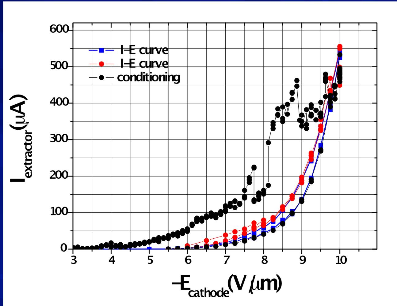
Maximum emission current : 550  $\mu\text{A}$  @ 2000V (  $E=10 \text{ V}/\mu\text{m}$  )
