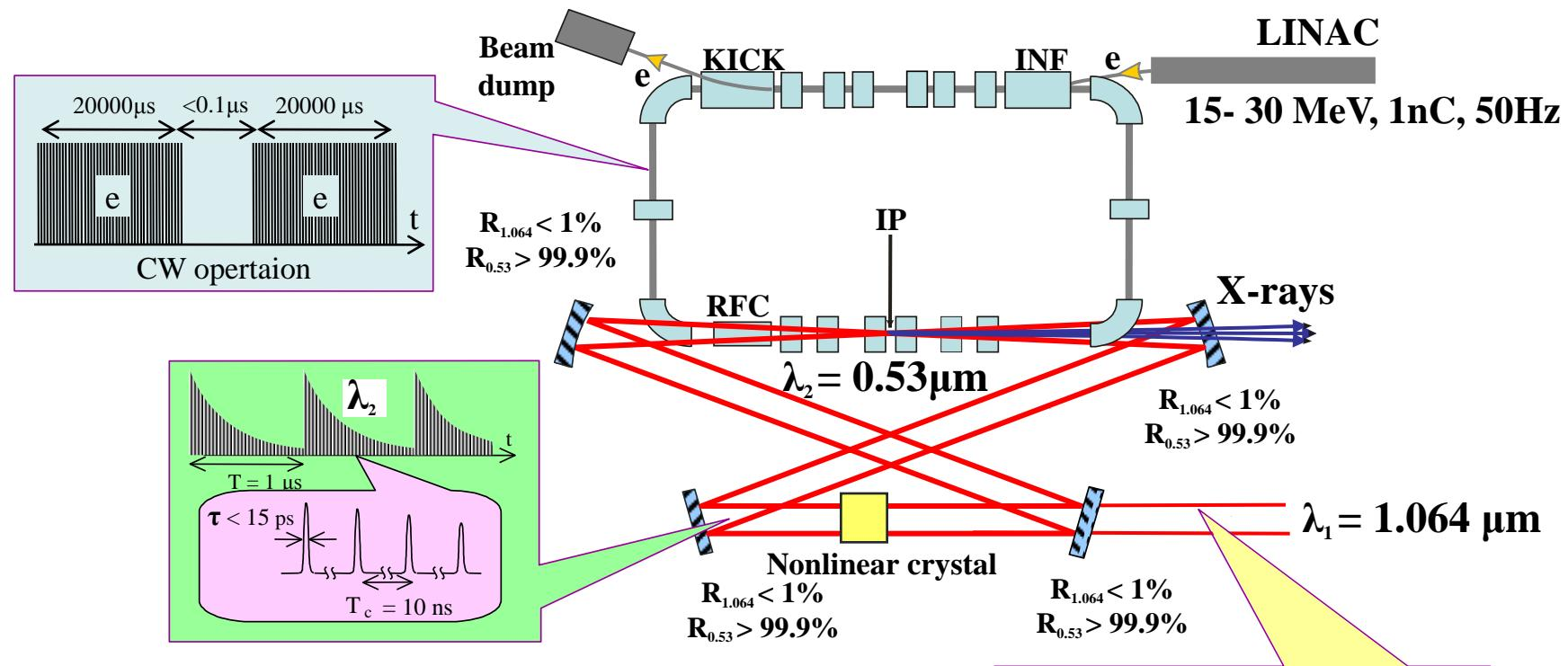
**CW Laser-electron X-ray Generator
