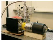
Fig. 2. X-ray source - Hamamatsu L9191 microfocusing X-ray tube.
