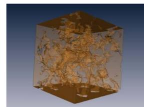
Fig. 10. 3D view of reconstructed sandstone microstructure
