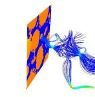
Fig. 11. An example of fluid velocity field obtained from LBM simulation (streamlines representation)
