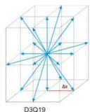
Fig. 5. Velocity vectors available in D3Q19 model
