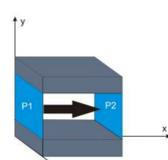
Fig. 6. Geometry of the Poiseuille flow between two parallel plates. Velocity profile in the y direction is parabolic
