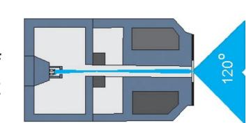
The radiation emitted from the source is focused on the sample with a use of the Rigaku multilayer mirrors in the Kirkpatrick-Baez arrangement. The Rigaku K-B mirrors are two ellipticaly curved multilayer elements perpendiculary fixed each to the other.
