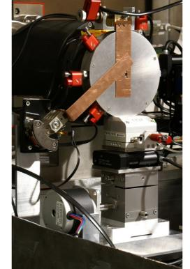
Due to the Bragg interference law, the radiation reflected from a multilayer is monochromatic, and the two multilayer elements of mirrors are optimized for 4.5 keV Ti K, line.
