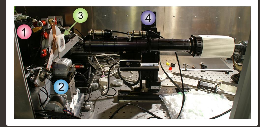
The optical microscope equipped with a camera and coaxial light source gives an image with the
