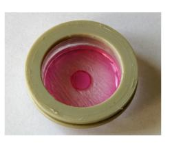
Cells are seeded and irradiated on 35 mm diameter Petri dishes with 10 mm round holes in the central part of the bottom. The bottom is covered with the 1.5 μm thick Mylar foil. A population of about 10<sup>5</sup> cells in 4 μl medium is seeded on the central part of the Mylar foil 16-18 hours before the experiments [4].
