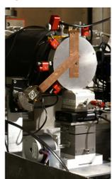
Beam shutter is a home made element. A half millimeter copper sheet is tighten to an old computer disk head driven by USB converter.
