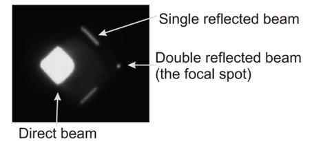
An x-ray could go through directly not touching the mirror (the direct beam), reflect from only one surface (the single reflected beam) or from both surfaces, which gives the doubly reflected beam which is the focal spot.
