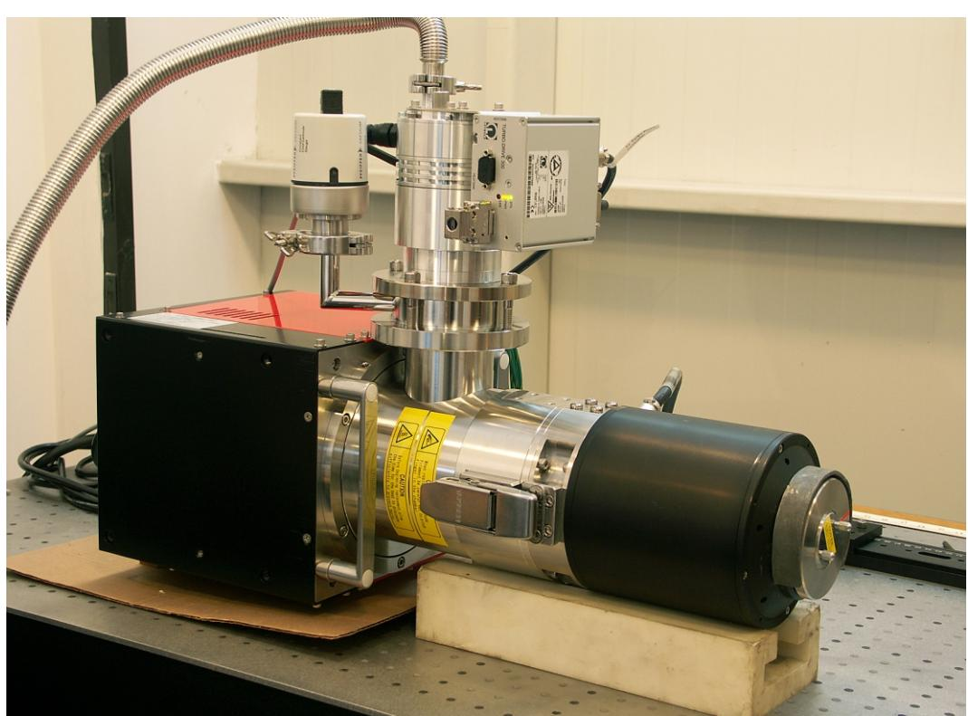
Voltage: 20kV - 160kV, tube current: 0 - 200 µA\*
